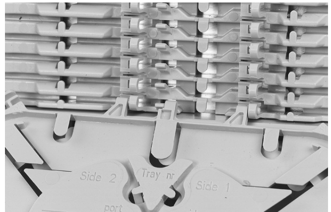
3.3 Place a tray in the wraparound groove plate; do this by pushing the lip on the groove plate (lowest possible position) slightly down with the tray and move the tray lateral into the hinge-cavities of the groove plate. To snap the High Capacity Single Element tray (HCSE) in the W/a single fiber groove plate leave always one hinge facility open between Fasblock or previous tray and the HCSE-tray.
